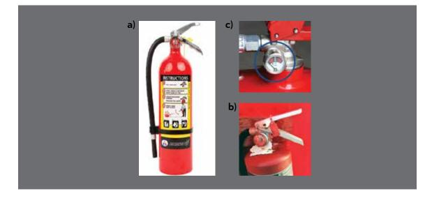
FIGURE 2: Fire extinguisher: (a) in good working condition, (b) defective, foam leakage and (c) defective, empty fire extinguisher
